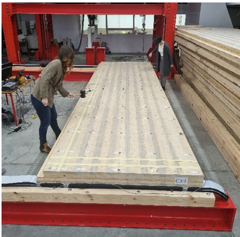
Figure 15. Modal testing of hybrid FRP-CLT panel
